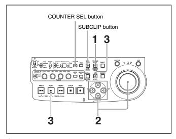
With the SUBCLIP button off, press the THUMBNAIL button, turning it on.
